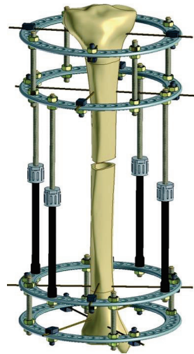
Figure 2. Full-ring circular external skeletal fixation system applied for tibia lengthening (Adapted from Zamani, A.R., Oyadji, S.O., Analytical modelling of Kirschner wired in Ilizarov circular external fixators as pretensioned slender beams, Journal of the Royal Society Interface 2009, 6:243-256)
