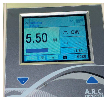
Figure 52. The parameters of the diode laser for ablation of the corneal tumour
