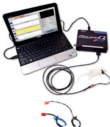
Figure 1. MouseOx Plus pulse oximeter used in mice for noninvasive physiological vital signs monitoring
