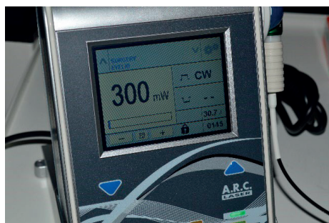
Figure 2. The parameters of the diode laser for eyelid surgery
