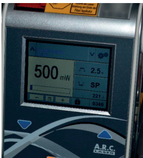
Figure 44. The parameters of the diode laser in transscleral surgery for glaucoma
