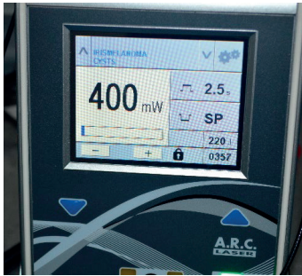
Figure 33. The parameters of the diode laser for uveal cysts surgery
