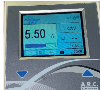
Figure 52. The parameters of the diode laser for ablation of the corneal tumour
