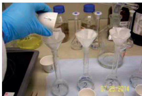
Figure 2. The ash was dissolved in 10 ml of dilute nitric acid. The filtrate was transferred quantitatively to a 100 ml volumetric flask and made up to the mark with distilled water
