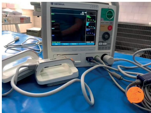
Figure 1. The D500 defibrillator from South Korean Manufacturers Mediana used for the experiment
